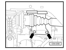
Unscrew nut -arrow- on both vehicle sides and remove coupling rods from the anti-roll bar.
