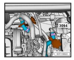
Unscrew screws-arrows- and remove ATF radiator.
