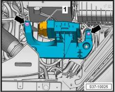
Unlock the catches -arrows- and remove the automatic gearbox control unit - J217- from the mounting bracket.
