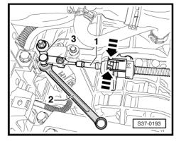
Unhook the selector lever control cable -1- from the clip -arrow- at the gearbox.
