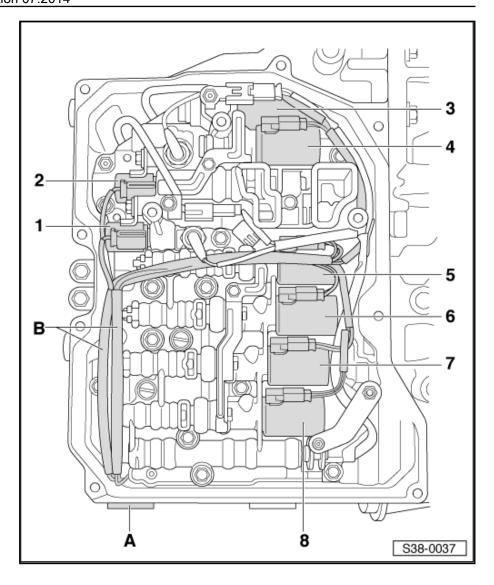
Make a sketch by hand in the same way as for the illustration with all the solenoid valves and their plug connections and mark all the plugs with the corresponding colour. Also mark the related cables with the corresponding colours.
