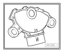
Fitting location: The multi-function switch is located at the top of the gearbox. The plug connection -5- is directly placed onto the multi-function switch.
