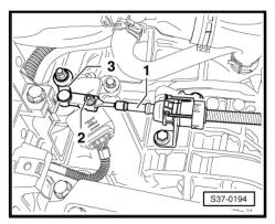
Hang the selector lever control cable -1- in the clip -arrow- at the gearbox. When installing the selector lever control cable, respect a minimum distance of at least 5 mm from the ATF cooler.
