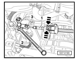
Unhook the selector lever control cable -1- from the clip -arrow- at the gearbox.
