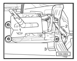
The fitting together of the plug connection -A- must not be performed, if the plug connector housing is latched into the shift mechanism. When fitting together (high resistance because of the spring) the catch of the plug connector housing breaks off.
