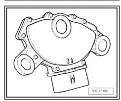
Fitting location: The multi-function switch is located at the top of the gearbox. The plug connection -5- is directly placed onto the multi-function switch.
