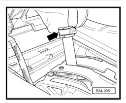
Detach the selector lever handle -1- together with the selector lever collar from the selector lever towards the top -arrow Aso that the lock button -2- is not pressed in.
