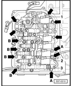
Wiring loom with 8-pin plug and integrated gearbox oil temperature sender - G93- -Arrow-
