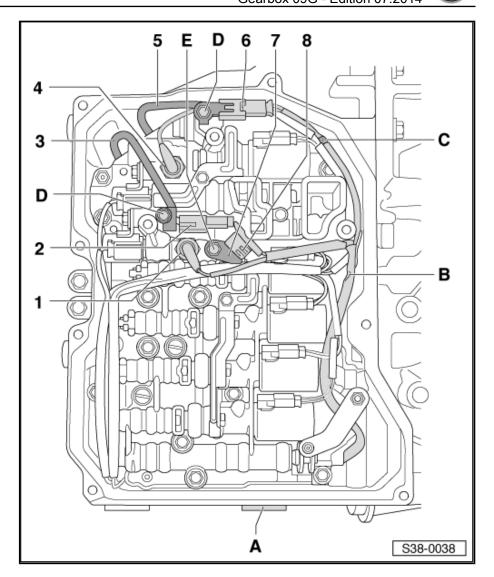
Unscrew the 3 screws -D- and -E-.Carefully disconnect the following plug connections:
