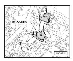
Remove the ATF radiator -1- from the gearbox -arrow A-.
