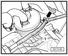
Removing and installing slave cylinder
