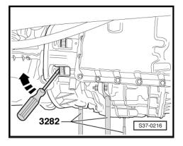
Prevent the torque converter from falling off, e.g. using a wire
